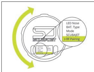
7 Open the main menu of both devices again and select **RF Pairing**. Confirm your selection by pushing the **righthand** button.
