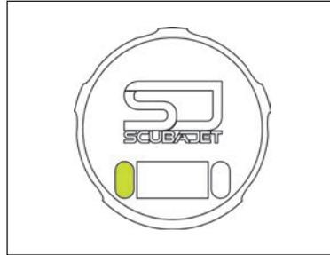
2 Turn on both the remote and repeater by pushing the **lefthand** buttons for **2 seconds**.
