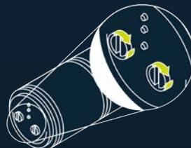
3 Only tighten and loose the screws on top of the battery by hand. Do not use a screw driver, but you may use a coin.
