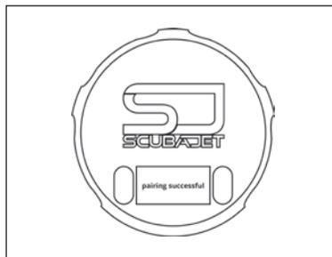
8 The pairing process starts once „REQ received” appears on the remote. Wait until **both** devices display „pairing successful”.
