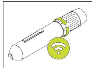
9 Turn the SCUBAJET control ring to **wireless** before using it.
