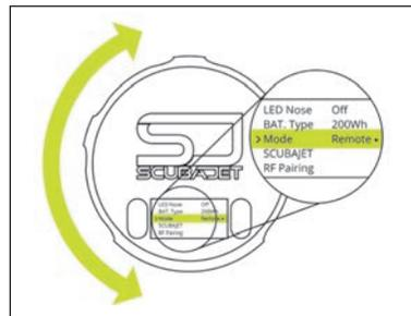
4 Turn the outer ring and select „Mode” in the main menu of the remote and repeater and activate „Repeat” and „Remote” mode on the corresponding device by pushing the **righthand** button.
